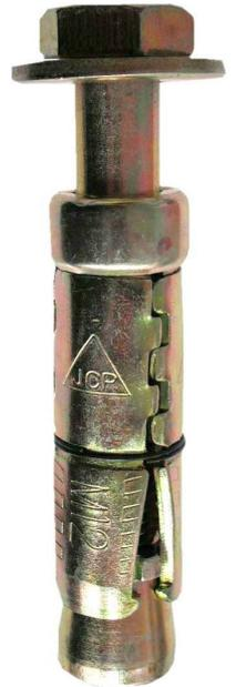
**PROJECTION BOLTS** Suitable for use in brick and concrete. The thick walls of the expanders give the anchor its exceptional grip & allows it to cater for oversized holes caused by powerful drills in weaker materials such as brick work.
