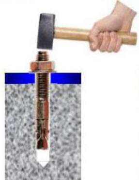
Insert assembled anchor through fixture into concrete
